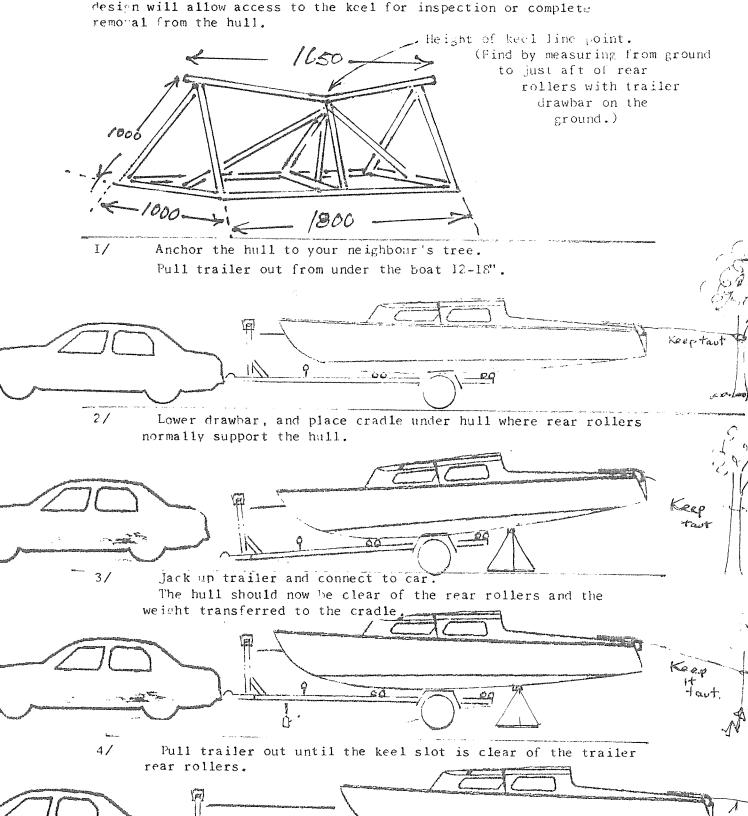
5/ Chock the trailer wheels. Fit two small stands under the rear of the trailer. Disconnect car and neighbour's tree. Keel may now be lowered to ground level.
